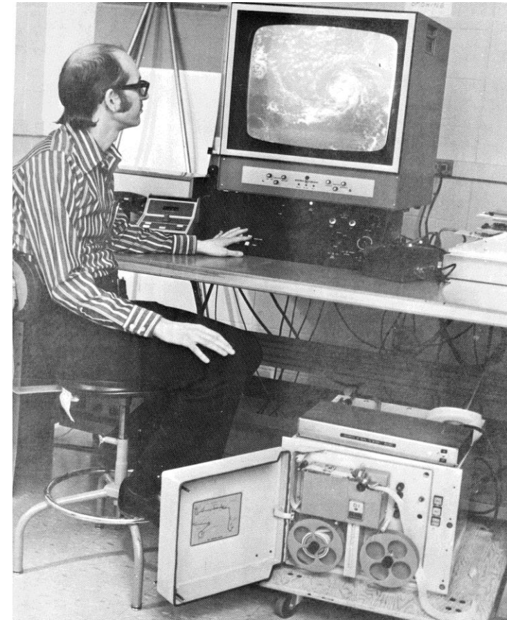
Man-Computer Interactive Data Access System (McIDAS) display
