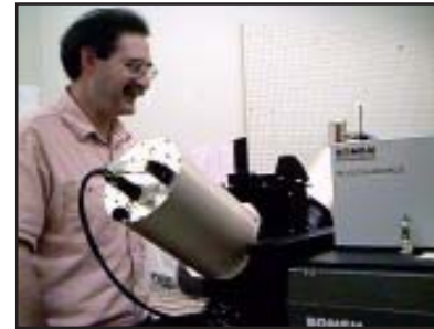
Fred Best with the AERI, a ground-based instrument in SSEC’s arsenal of instruments to study the atmosphere.
