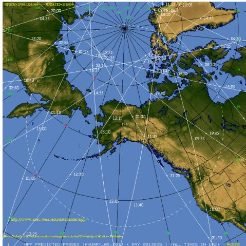
Suomi NPP daily orbit track and antenna coverage using GINA site as an example. Direct broadcast acquisition and CSPP VIIRS product generation provides timely data delivery to National Weather Service WFOs.
