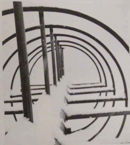
LIKE A GIANT corkscrew, the antenna (ABOVE) rotates a complete 360° and can be raised 90° from horizontal. When installed, it received data from ESSA VIII and Nimbus IV weather observing satellites.
