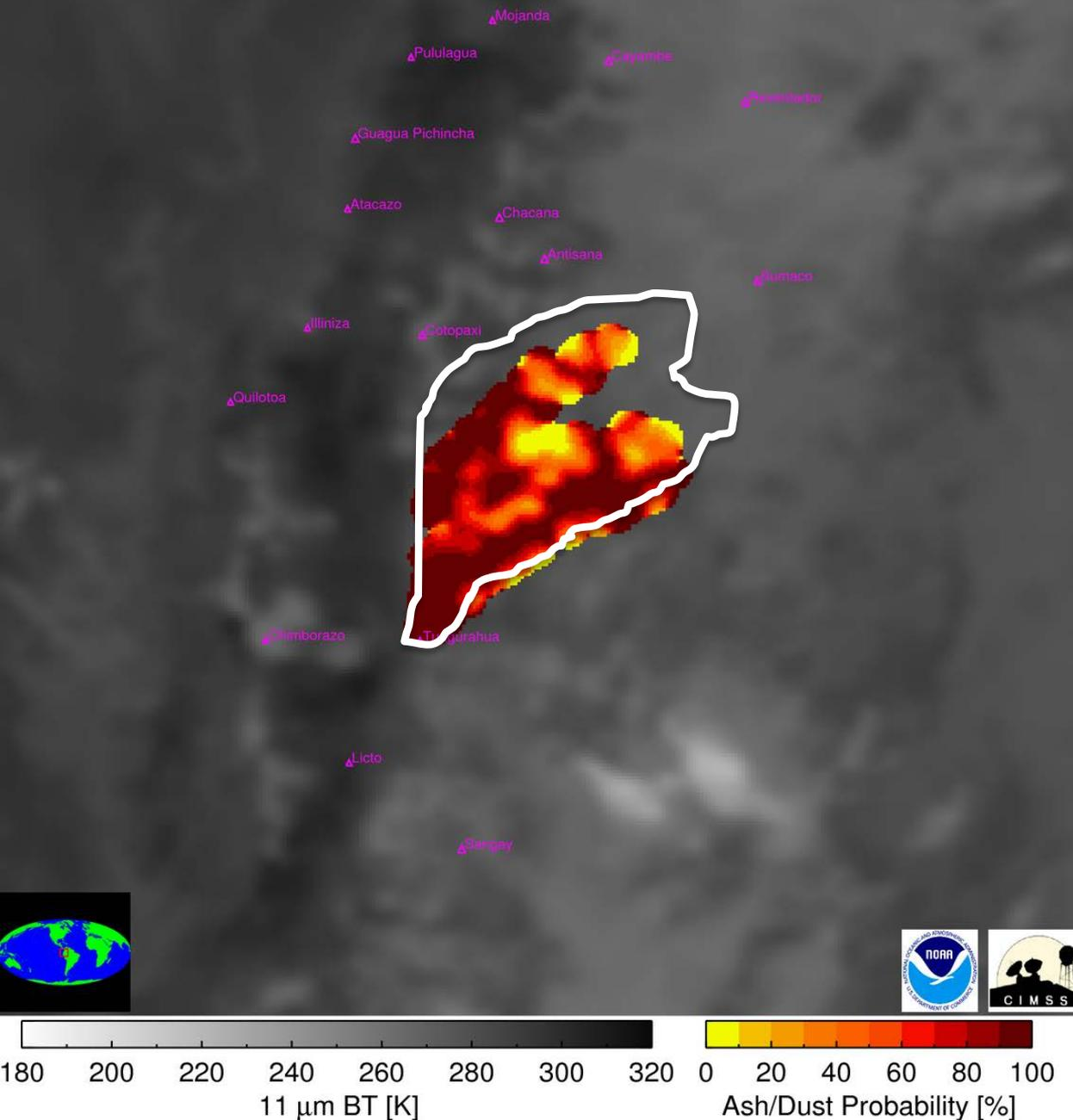
The horizontal extent of the ash cloud determined by GOES-R/JPSS automated computer algorithm agrees very well with the bounds derived from manual analysis of multi-spectral imagery
