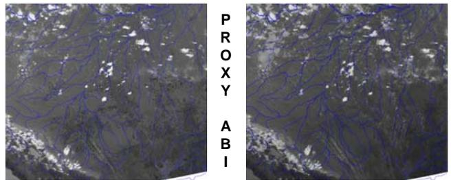
The initial iteration of the WF\_ABBA for ABI takes the 3.9 μm and 11 μm bands to perform its detection and characterization. The fire mask below contains cloud information (white), regions not processed for various reasons (black), the regions processed (dark green), and categorized fires (various colors):
