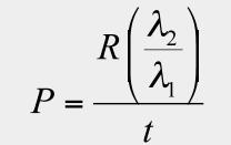
R = spectral resolution  $\lambda_2 = \text{longest wavelength in FSR}$  $\lambda_1$  = shortest wavelength in FSR t = time to S/N=10 Å<sup>-1</sup> for  $H_{AB} = 19.5$
