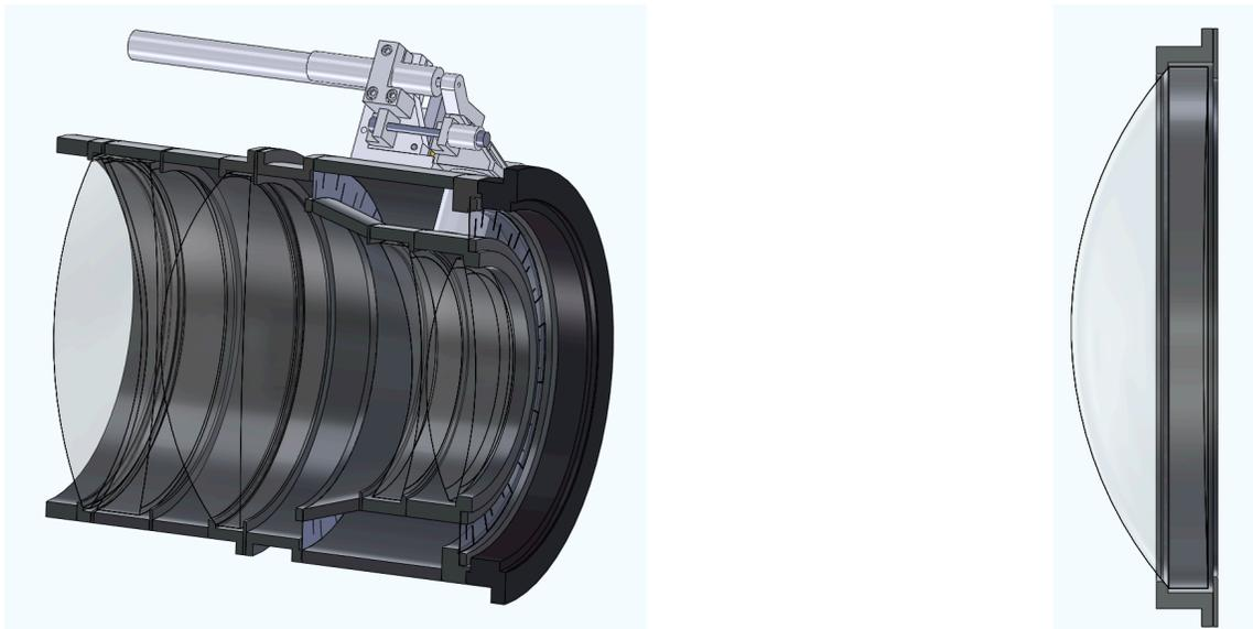
**Figure 5-28. a.** Cut view of camera barrel showing diaphragm flexure mounting of element 4 and 5. **b.** Single element mounted in its cell showing tangential shoulder and ~2mm elastomer gap.
