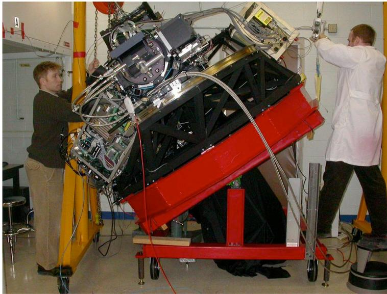
**Figure 6-2.** *RSS-VIS shown in its flexure test and integration platform. RSS-NIR will use a similar platform but will have the ability to vary the azimuth angle.*
