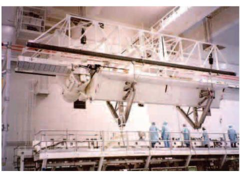
Engineers at the Kennedy Space Center maneuver the main antenna onto a workstand.
