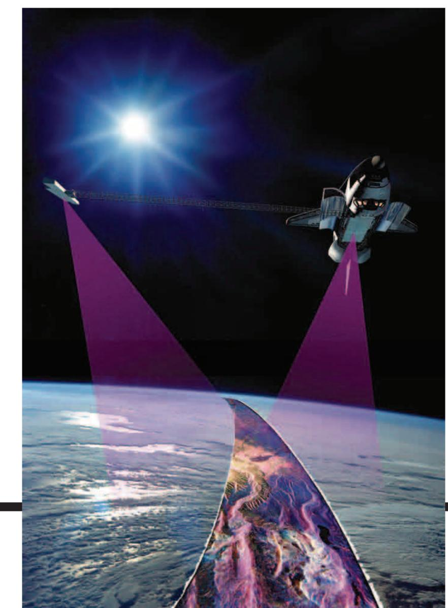
Artist's rendering of Space Shuttle Endeavour mapping the topography of Earth, from some 145 miles (233 kilometers) above with SRTM radar instruments. Unlike most optical sensors, radar is capable of "seeing" through clouds and at night.
