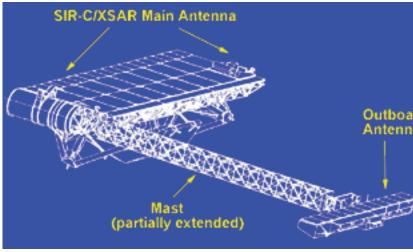
The SRTM instrument was made up of three sections: the main radar antenna, the mast, and the outboard radar antenna. Credit: NASA
