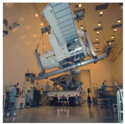
Joining the SRTM outboard antenna and mast canister (foreground) with the main antenna (background) at the Kennedy Space Center Multi-Payload Processing Facility. Credit: NASA
