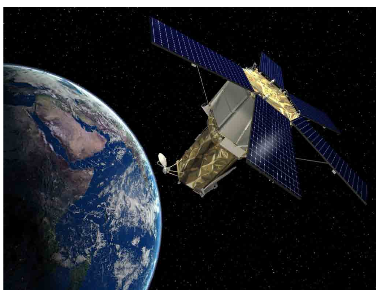
Artist's drawing of GeoEye-2. Its launch is planned for early 2013. It will be capable of 10in (25cm) resolution imagery but access will be restricted. Credit: GeoEye
