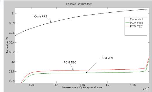
Early results show CORSAIR cell temperature sensors consistent with known melt points to within ~20 mK. Temperature sensors were calibrated to ~15 mK (1σ) prior to placement in blackbody
