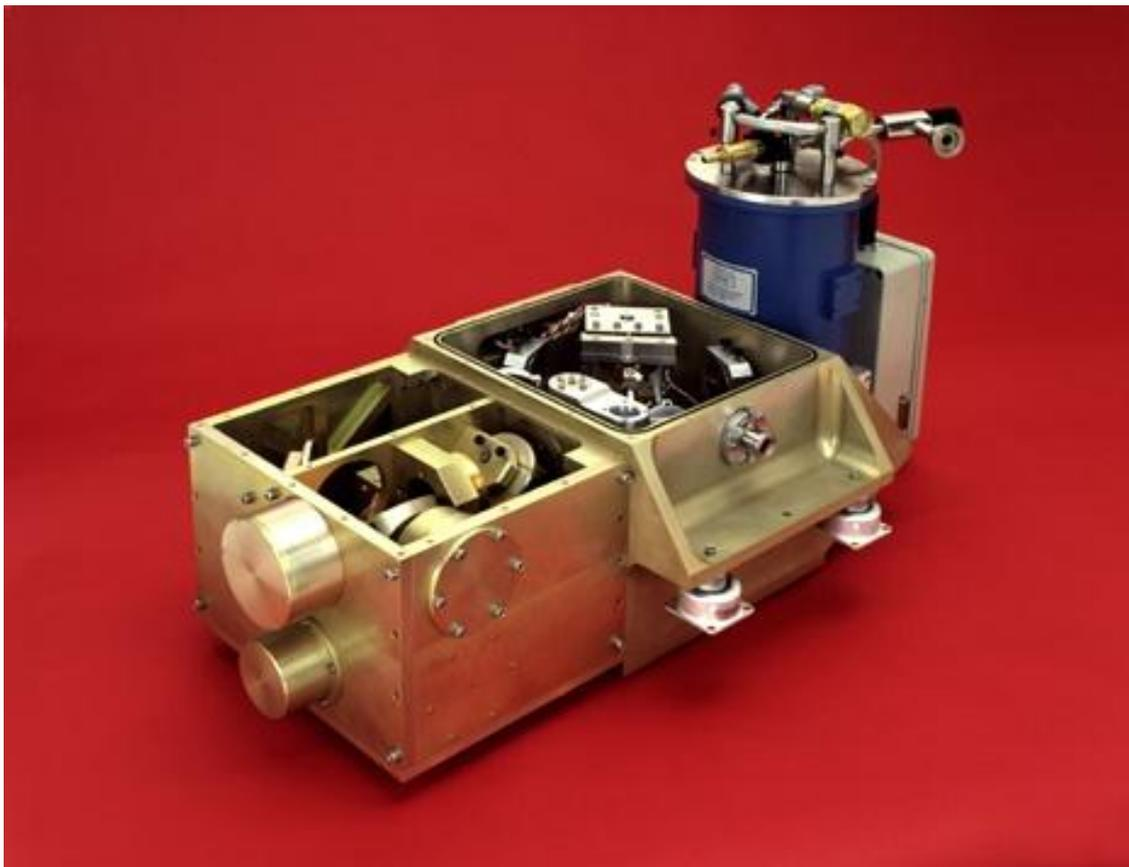
4-port polarising interferometer employing thin film beamsplitter and helium cooled detector.
