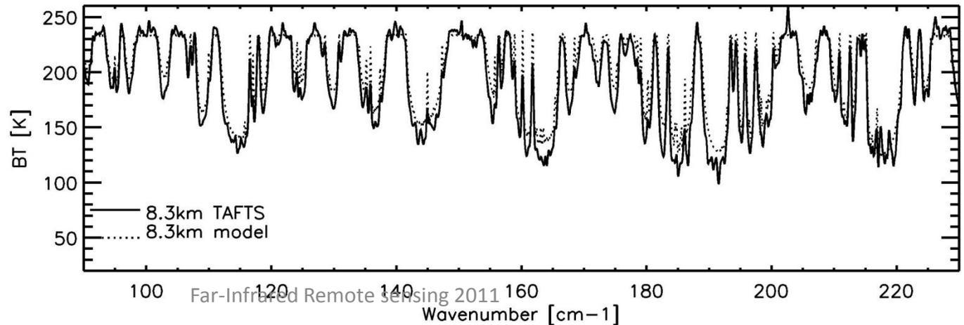
The FIR variation observed across the FL track is limited by that of the measurement uncertainty, however, the model deviation (derived from the meso-scale atmosphere variation) should be just discernible.
