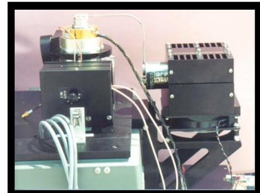
**Detector with Stirling Cooler**
