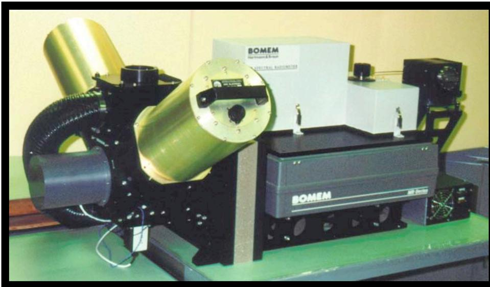
**Interferometer Assembly with Blackbodies**
