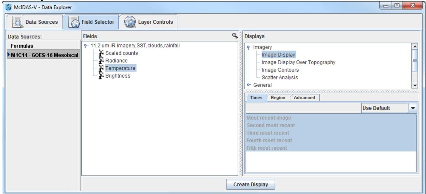
The **Field Selector** tab analyzes the data source to determine the displayable fields and parameters. With this information, a list of available displays is presented. In the **Subset** panel of the **Field Selector** there are tabs to select which times to display, which region to use, as well as a variety of advanced options. Note that the tabs in the **Subset** panel will differ dependent on which data source you loaded.
