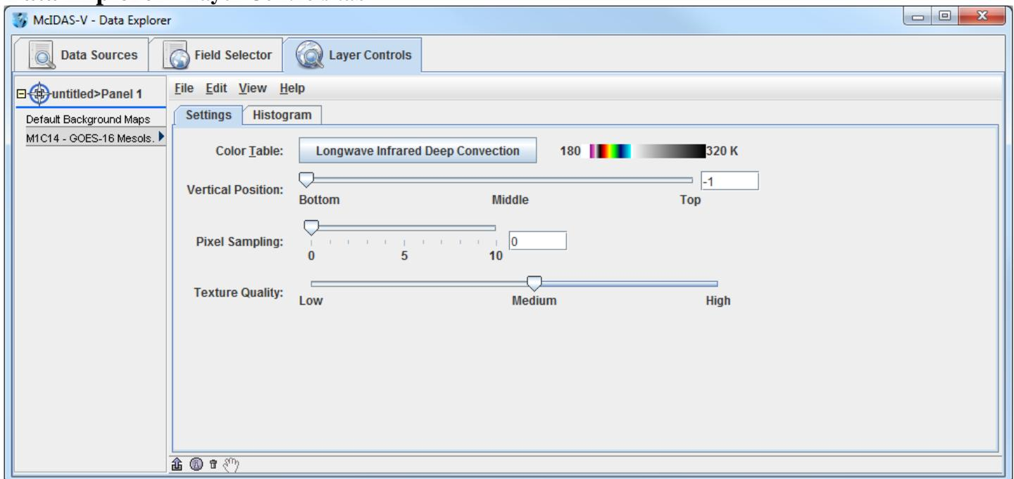
The **Layer Controls** tab contains the display options for the displayed fields and parameters which are referred to as layers. Changes made to each layer will be reflected in the **Main Display**. Also, if a graph, time series or special display was selected, it will display in the **Layer Controls**.
