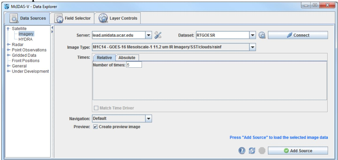
The **Data Sources** tab is used to locate remote data servers or local files for display in McIDAS-V. Once the type of data source is selected, a chooser with the appropriate selection criteria is displayed. **Satellite -> Imagery** is chosen above, and the **Satellite -> Imagery** chooser is displayed. Other data source types are the HYDRA multi-spectral display, Radar, Point Observations, Gridded Data and General files.
