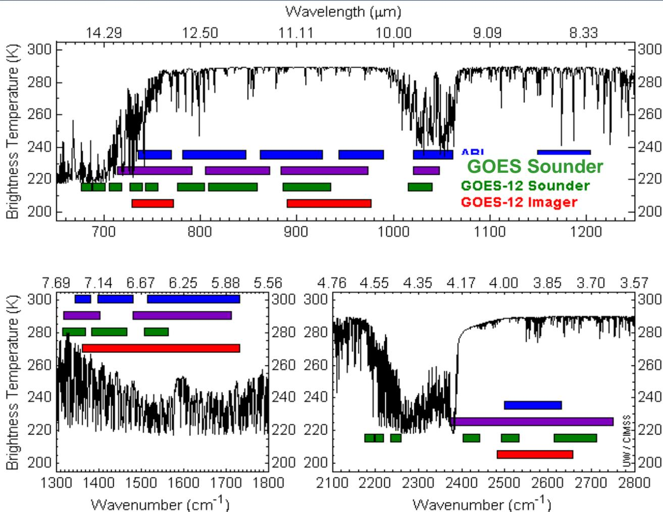
ABI (blue) and current GOES sounder (green) spectral coverage over a high spectral resolution brightness temperature spectrum.
