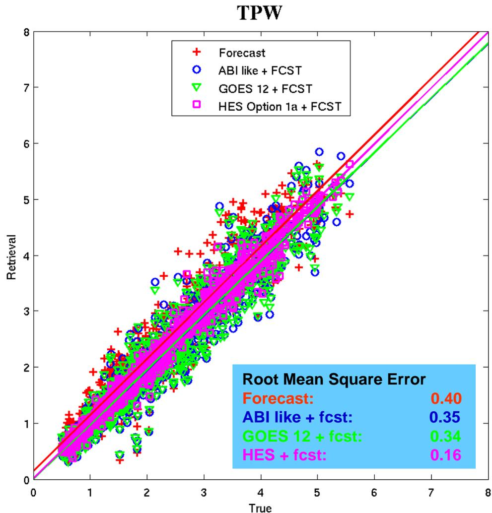
Experiments show that retrievals of Total Precipitable Water (TPW) from high-spectral (e.g., HES) data are much improved over current broadband (GOES-12+forecast).
