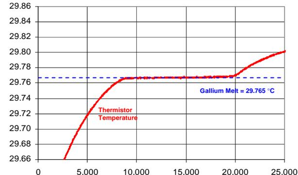
Melt Signatures Provide Absolute Temperature Calibration Accuracies better than 10 mK for full atmospheric Temperature Range
