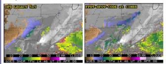
SFOV products tend to be spatially less smooth than larger FOV products (shown is 5x5 FOV; 3x3 would be similar but with slightly better resolution), especially near and adjacent to clouds. Retrievals of TPW are heavily dependent on the accuracy of the underlying cloud mask.
