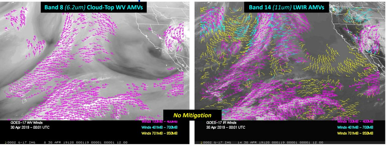
Reductions in AMV counts and quality occur when the ABI Focal Plane Module (FPM) temperatures are too warm (approx. 10:00 – 15:00 UTC here). High level winds, derived from tracking optically thin cirrus targets, suffer height assignment issues when the 12 and 13.3 um bands are degraded or saturated.
