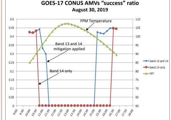
Time series showing example of the impact of adding band 13 as a mitigation across a period of maximum FPM heating.
