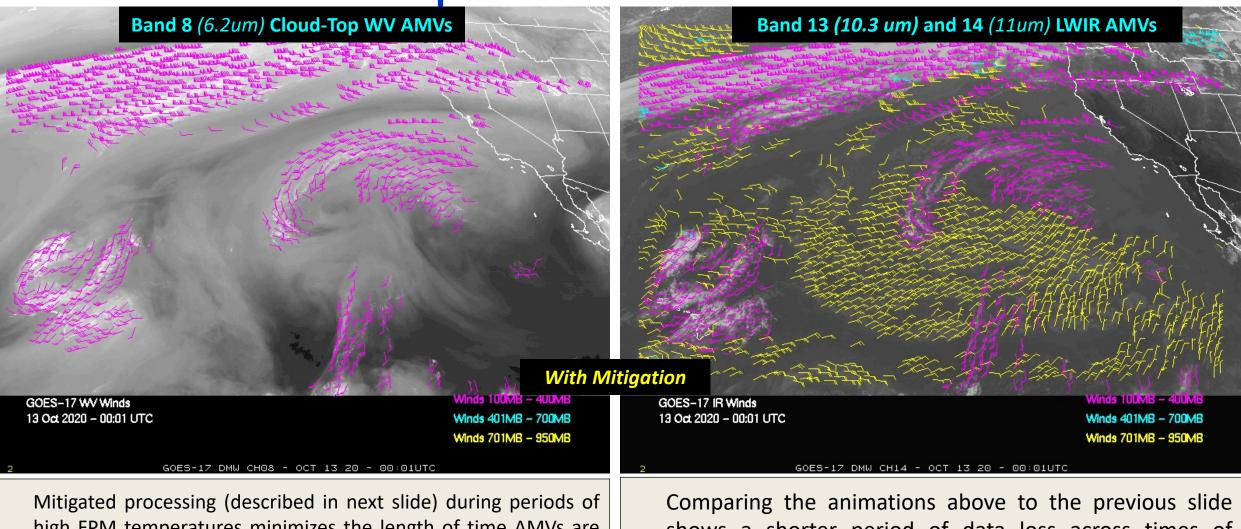
high FPM temperatures minimizes the length of time AMVs are impacted. (Note: animations above are from a different, but comparable, FPM warm period than previous slide) Comparing the animations above to the previous slide shows a shorter period of data loss across times of greatest heating (approx. 10:00 - 15:00 UTC here). See time series plot in next slide.
