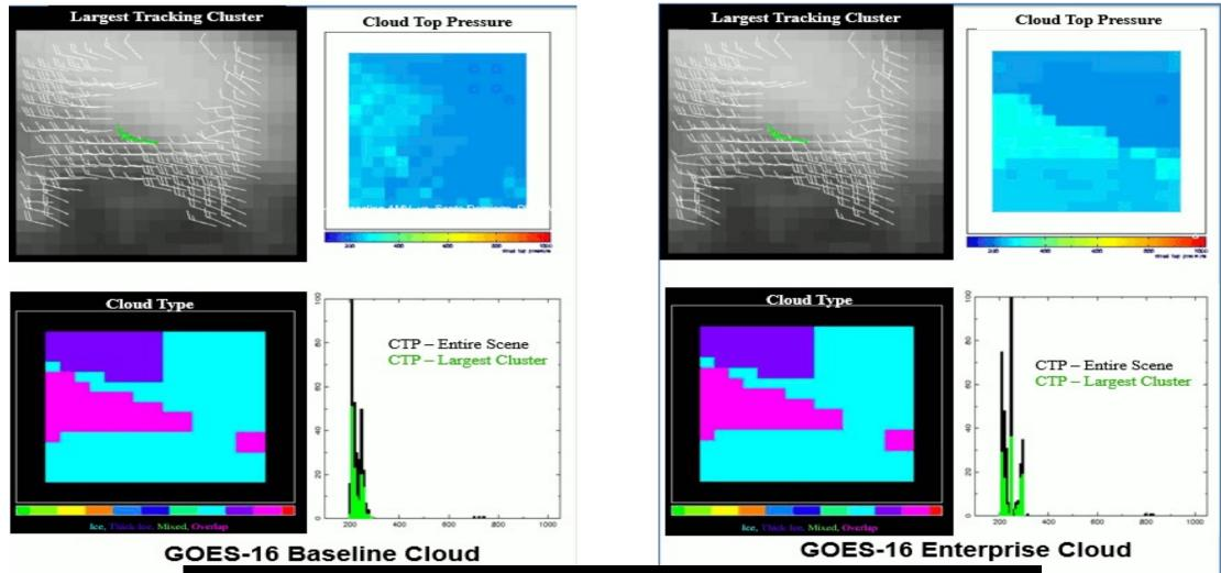
The Enterprise algorithm more accurately resolved the structure of the multilayer scene as shown here in the respective CTP histograms and CTP plots of the target scene.
