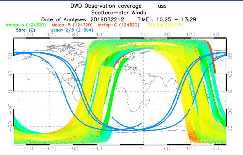
Operational scatterometer: ASCAT-METOP A/B/C and ScatSat, Monitoring HY-2A/B Operational altimeter: Jason 2/3 and SARAL Monitor: Sentinal A/B
