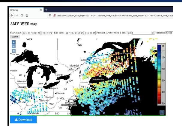
A WFS webmap application. Data are directly queried from the PostGIS database via Geoserver. Filtering possible by dataset, variable, height level, and quality level. Performance improvements to be expected by raster representation of AMVs and pre-tiling. Quick analysis tool of AMVs, including data querying and export. Overlay of multiple datasets for collocation studies.
