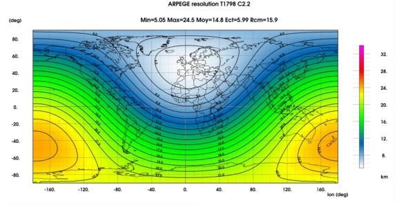
Spectral model with variable resolution:  $T_{L}1798c2.2L105$
