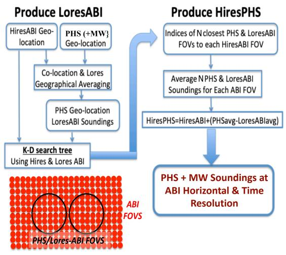
(1) The first step of the fusion process is to spatially average the high horizontal resolution ABI soundings to the footprints of the CrIS and IASI polar hyperspectral sounding instruments. This provides a paired low-resolution ABI and coincident polar hyperspectral sounding training data set to be used to predict polar hyperspectral soundings at the locations and times of every full resolution multispectral ABI data point.
