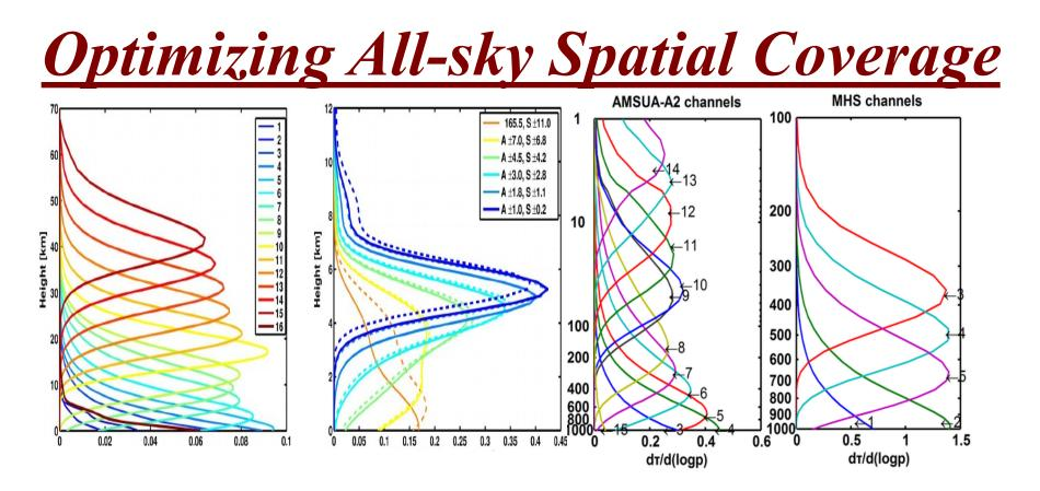
ATMS: Vertical Res. 5-10 km H<sub>2</sub>O Horizontal Res. 15-km Time Res. Same as CrIS AMSU/MHS: Vertical Res. 5-10 km H<sub>2</sub>O Horizontal Res. 15-km Time Res. Same as IASI
