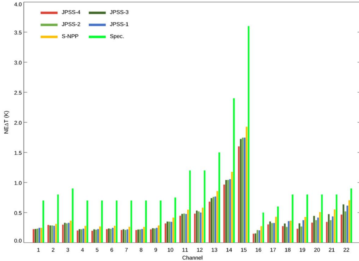
Comparison of 22 channel NEAT of all JPSS builds indicating all channels meet the design requirement and improved channel sensitivity in future JPSS ATMS builds are expected
