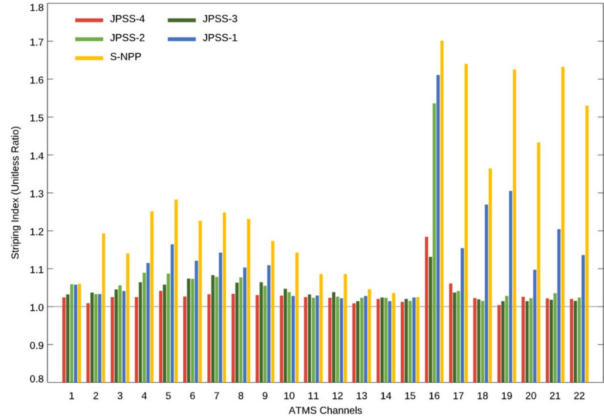
Comparison of 22 channel striping indices of all JPSS builds indicating a reduced channel striping effects in J2/3/4 ATMS
