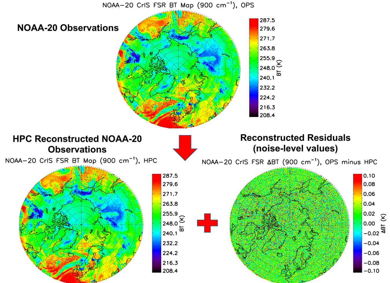
(Top) NOAA-20 CrIS Observations. (Bottom) NOAA-20 CrIS HPC reconstructed observations (Bottom-left) along with reconstructed residuals (Bottom-right) over north pole for 14 Dec 2021. The application of HPC compression is expected to provide significant data compression (more than one order of magnitude).
