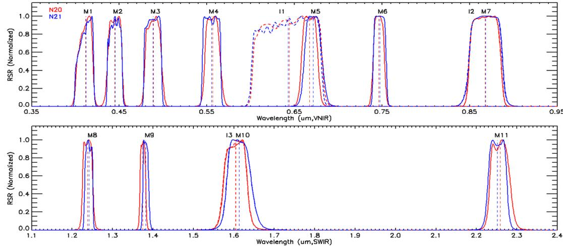
**Figure 1.** Comparison of NOAA-21 (N21, blue) and NOAA-20 (N20, red) VIIRS solar band Spectral Response functions
