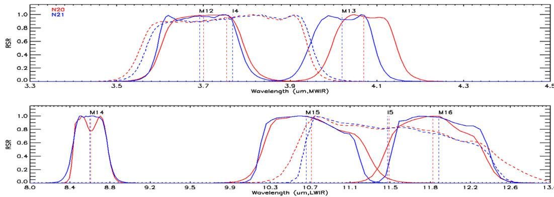
Comparison of NOAA-21 (N21, blue) and NOAA-20 (N20, red) VIIRS thermal band Spectral Response functions
