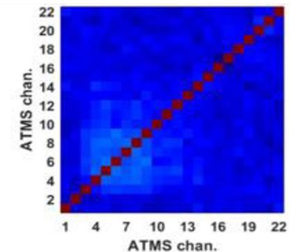
Example of SNPP ATMS analysis showing large channel noise inter-correlation that degrades application performances. NOAA-20 ATMS intercorrelation is reduced. J2 ATMS inter-correlation is further improved, particularly for water vapor channels ( Ch. 18 – 22).
