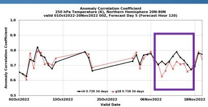
500 hPa geopotential height ACC scores are neutral in both hemispheres 200 hPa mean vector wind expresses a significant negative bias in the tropics A forecast dropout period appears in November without a known cause
