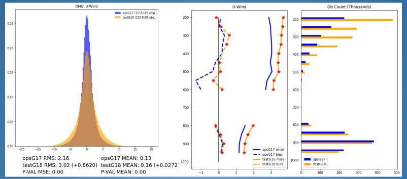
**Initial tests** of GOES-18 AMVs, monitoring OmB statistics without assimilation, showed a **significant RMS increase** relative to operational GOES-17 AMVs. These departures were **not** present during cycled assimilation tests performed later.
