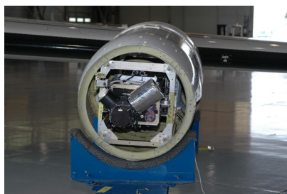
Scanning High-resolution Interferometer Sounder (S-HIS), SSEC's airborne instrument measuring temperature and water vapor profiles.
