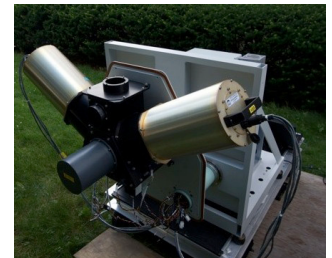
Atmospheric Emitted Radiance Interferometer (AERI), an advanced, ground-based version of the high-spectral resolution interferometer sounder.
