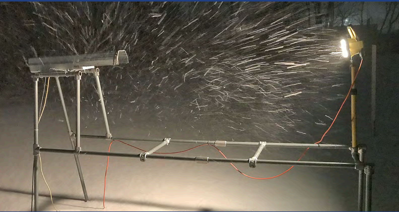
▲ A ground-based instrument called the Precipitation Imaging Package provides information about precipitation characteristics that can help improve estimates of snowfall rate and accumulation. It is shown here collecting measurements during a snowstorm at an observational site near Marquette, Michigan. Credit: Mark Kulie
