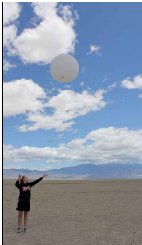
UW AOS students Jacola Roman and Elise Garms launching and tracking a Vaisala radiosonde.
