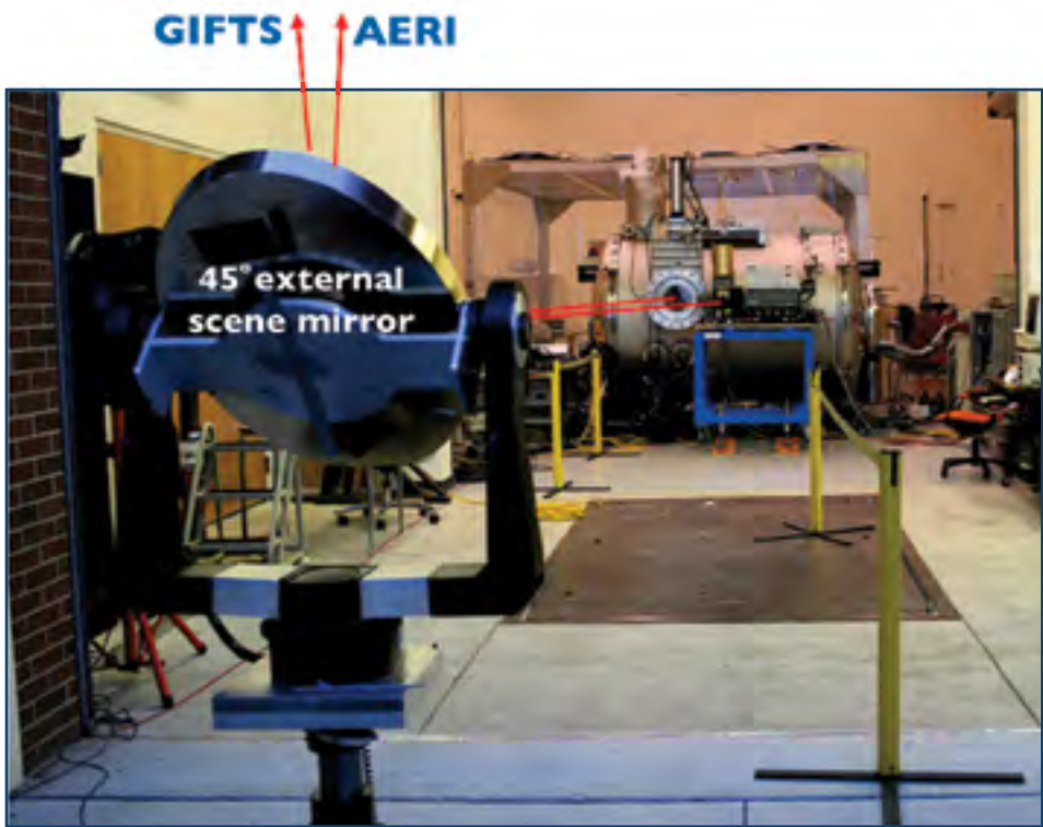
Figure 2. Zenith sky viewing configuration showing the GIFTS chamber and view port with AERI sitting along side (blue rectangle is AERI cart). The radiance intercomparison includes about 40 feet of horizontal path.
