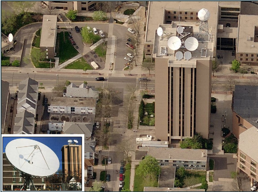
Figure 2. SSEC rooftop image showing the antenna systems that receive satellite and other data. An additional 11m dish is located on the ground 1 block to the south.
