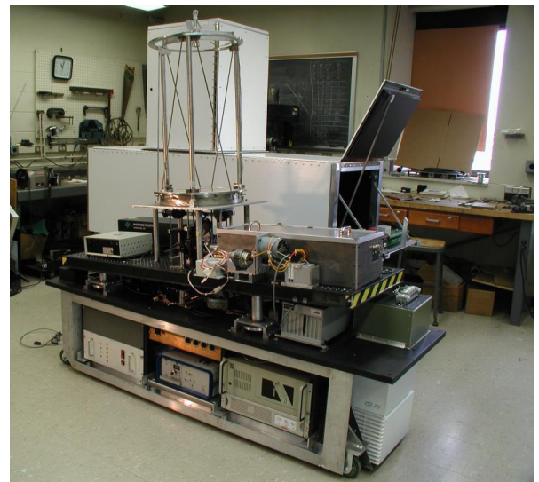
The LIDAR with the environmental housing removed.
