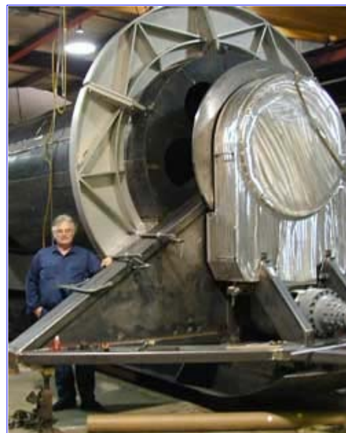
EHWD Hose Reel fabricated at UW–Madison's Physical Sciences Laboratory
