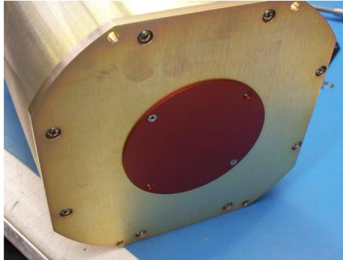
*Figure 4- 13. Remove red cover (4 screws)*
