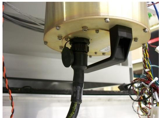
*Figure 4- 14. 2 Blackbody cable connections*
