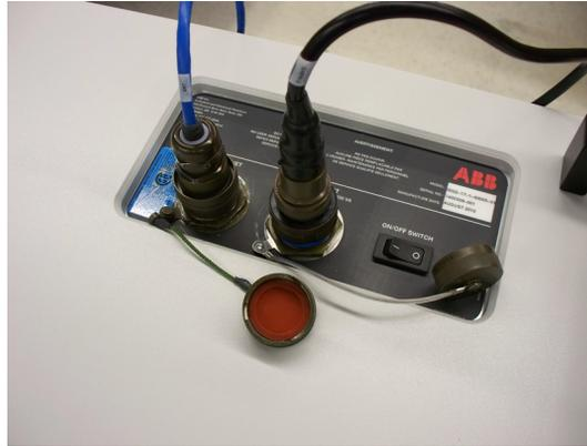
*Figure 4- 7. Connect Power cable*
