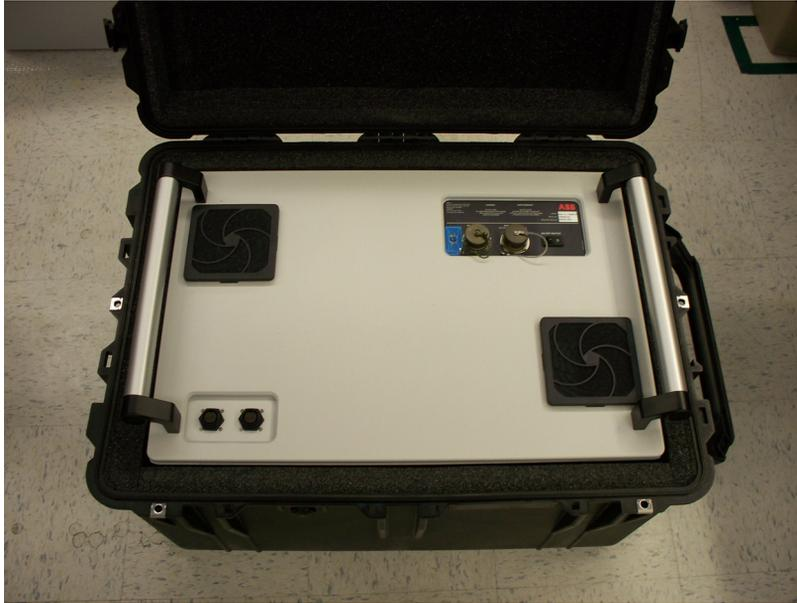
*Figure 4- 1. Blackbody Control Unit in its transportation box*
