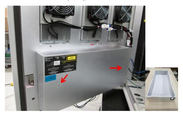
3. Remove the power supply and TEC controller cover (12 screws), this stainless steel cover has 12 screw that are mounted with an O-ring to facilitate the replacement of the panel. Pay attention to the cables on the right side when taking it out.
