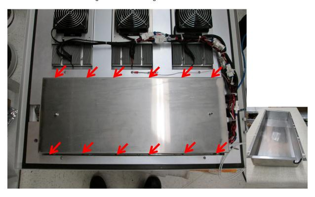
4. Once the Power supply and TEC cover removed, you will have access to the power supply and the TEC controller. This view show the door removed from the main frame. Don't take off the door.
