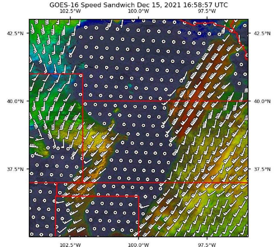
GOES 16 Ch 02 0.64  $\mu$  m imagery plotted with optical flow winds (white barbs) and the speed sandwich product over a strong low pressure system in the Central Great Plains.
