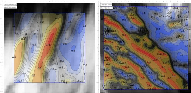
Example of actual correlations surface calculated during AMV derivation. The left figure is for a target box size of 15, and the right figure is for a target box size of 5. The correlation surface near the peak can be approximated by a parabolic fit, but its axis is generally inclined in a discrete direction and is not related to the target box size.
