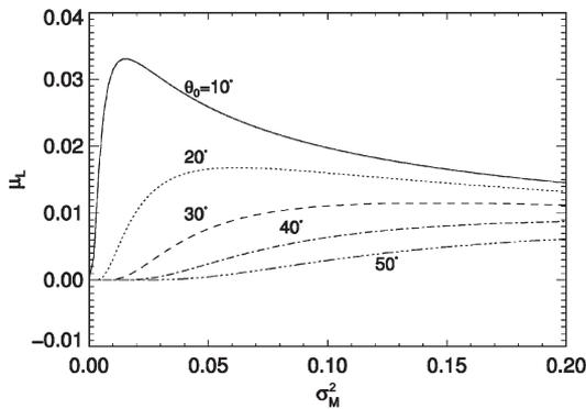
Fig. 9. Theoretical relationship between the glint mean and slope variance (21), for several solar zenith angles.
