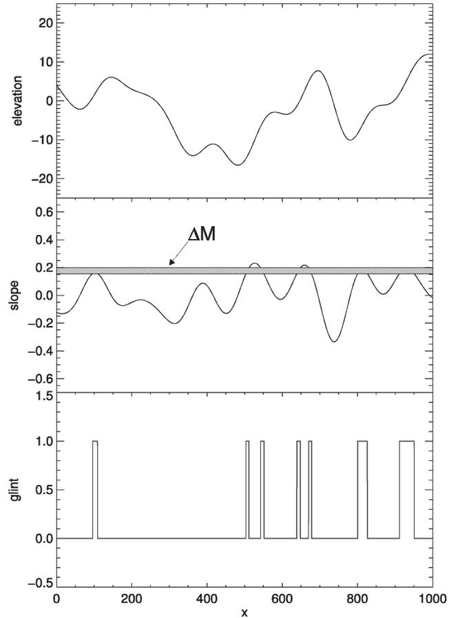
Fig. 2. Schematic representation (in arbitrary units) of the surface elevation  $\eta(x)$ , the surface slope  $M(x)$  with the slope range  $\Delta M$  selected by the glitter function, and the glint process  $L(x)$ .
