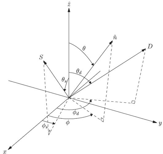
Fig. 10. Geometry of the specular reflection of sunlight from the ocean surface.
