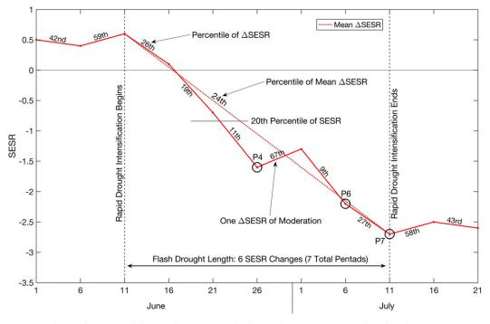
FIG. 2. A time series schematic illustrating the four criteria used in the flash drought identification methodology.
